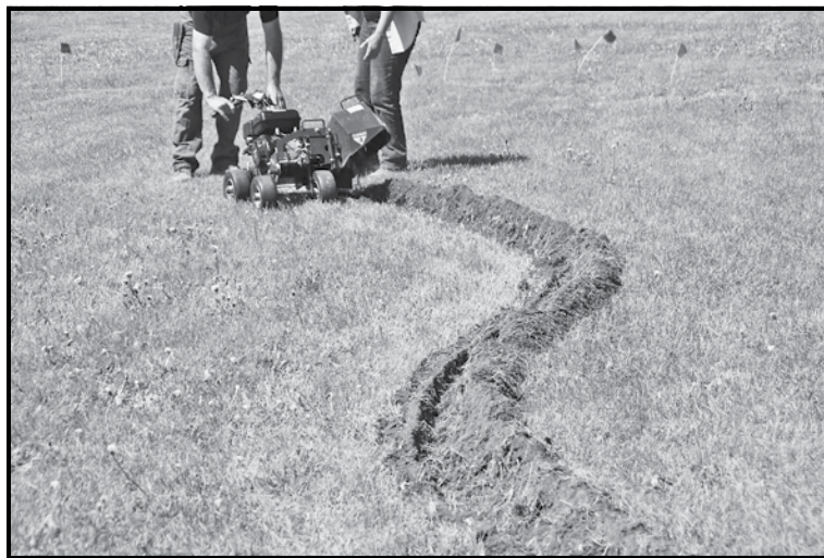
When creating large garden beds, rent a power edger to make the job easier.
